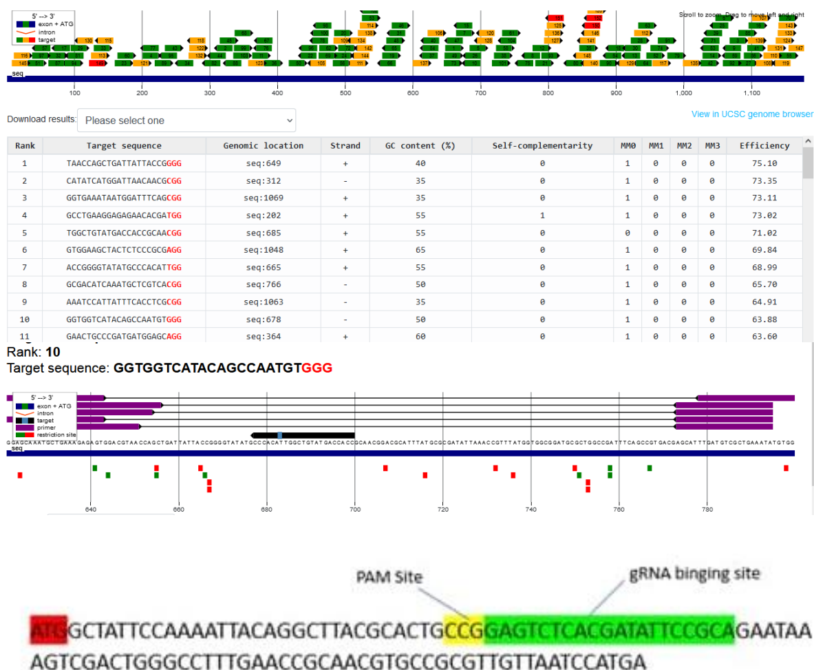
Fig 1. gRNA Examples from the CHOPCHOP Database for Use in Study and a Schematic Representation of the gRNA Binding Site and PAM Sequence in the entB Gene
